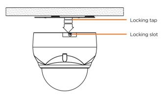
6. Fix the locking screw to secure the camera to the bracket and complete the installation.
