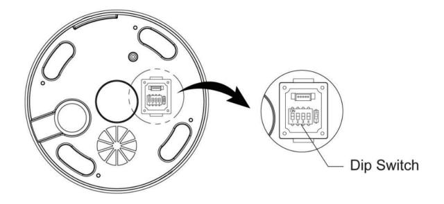
Control the camera's video signal and video type using D1 and D2, respectively, in the S1 switch.
