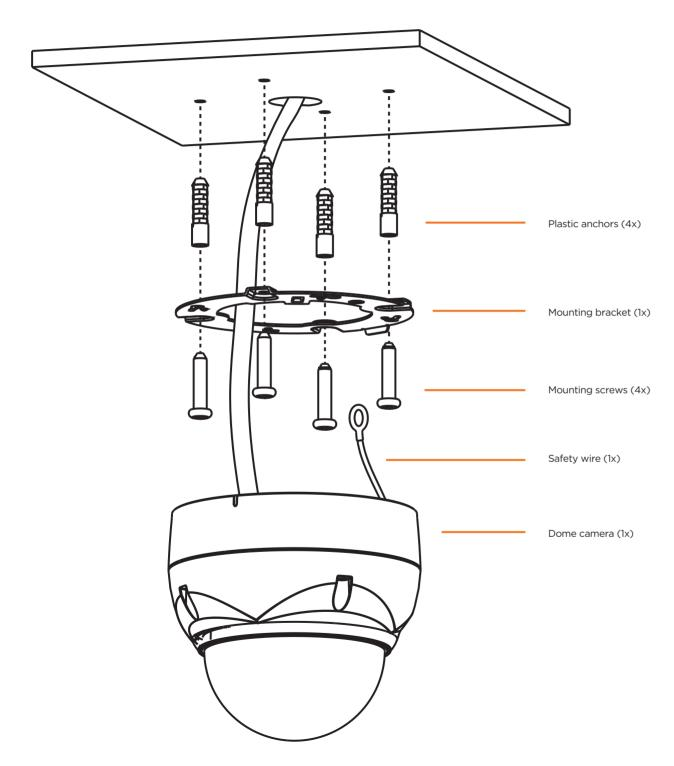
1. Using the camera or mounting template, mark and drill the necessary mounting holes in the mounting surface.
